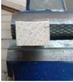
Best I DO NOT forget to drill holes in the bridge for the tie-on strings before gluing on!! With trial and error, I determined the angle of the hole had to be 10 degrees, so I cut a small block with that angle on one face. Maybe it's not obvious here, but the hole has to "rise" as it passes through, otherwise you'd be drilling into the plate on the other side. That is only a 3/32" bit - looks larger here.
