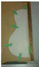
The 1/8" thick template is used to draw an outline on 2 pieces of 3/4" thick plywood and they are rough cut with a jig saw. The template is then double side taped to the plywood and the router table is used to shape the plywood into 2 identical form halves.
