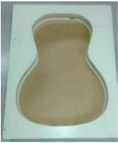
Hard to see the white pencil mark but it denotes the orientation of the sides where they (hopefully) will meet at the lower bout. I say hopefully because if you don't orient one of them correctly when you bend the sides, there goes the match of the grain at the ends.
