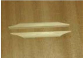
The full set for the top. Note that the x-braces are notched out so that they can cross each other. In between is a 4mm thick x-brace plate.
