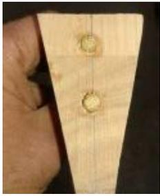
Decided to add a headstock plate of Black Walnut; here's where I marked off 1/16th of an inch to take off, then glue a plate on that's equal to the thickness that is removed. This plate will be visible in the next pic.
