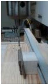
After removing the tape that covered the bridge area (so that I would not have to remove any finish) I made a last minute check for location accuracy. Seemed spot on, so I taped around the outer perimeter. This helps to locate the bridge when glue is applied and keeps glue off of the finish. After clamping down and removing any squeeze-out I removed the outer tape and there she'll sit overnight.
