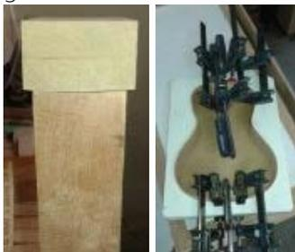
Time to glue on the back braces in my go-bar deck while the blocks dry.
