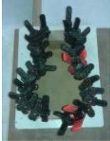
I routed a channel down the back seam on the outside (you'll see why in a later pic) so this will add strength to the seam. These don't go all the way to the ends because of the head and tail blocks.
