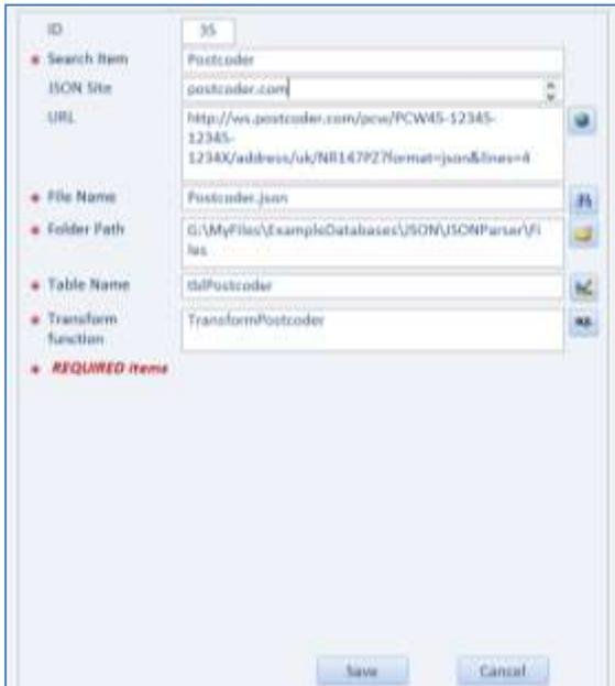
If using an online JSON source, click the **Get** button to save the data to the specified **.json** file
